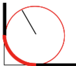
Rounded using an arc of circle
